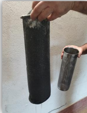
Filtering sock removal and substitution
